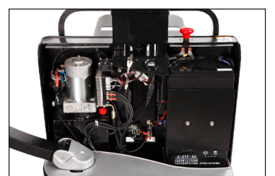
Built-in charger and maintenance free batteries
